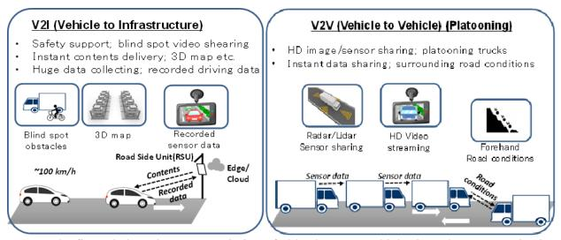
The figure below shows transmission of video between vehicles in a platoon organization using WiGig transmissions. Video sharing with low latency among platooning trucks is one of the use cases that can cooperatively utilize the 5.9 GHz band V2X as control channel.
