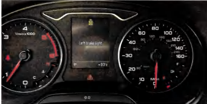
Figure 2: Indicator that left rear brake light is inoperative
