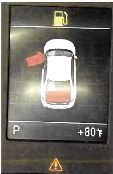
Figure 3: Indicator that left rear brake light is inoperative
